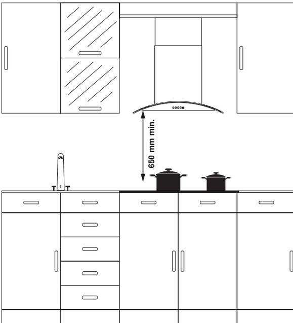
Product is designed in accordance with the kitchen counters supplied from market. A safe distance should be left between the product and kitchen walls and furniture. If hood/aspirator will be installed over your appliance, obey to the recommendation of hood / aspirator manufacturer for assembly height. (min. 65 cm)
