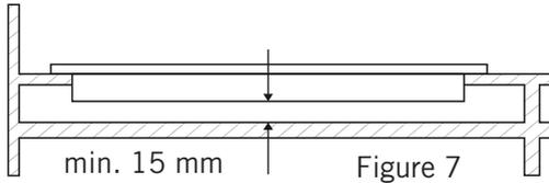
6. While mounting cooktop on a closet, as shown in the figure above, in order to separate between closet and cooktop, a shelf should be mounted. If it is mounted on a built-in oven, there is no need to do that.
